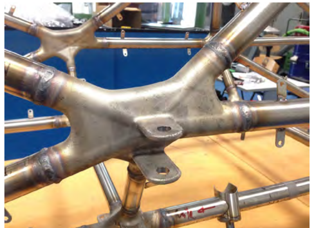
Close-up view of an assembled car frame section showing a four-way joint with integral hard point connectors
