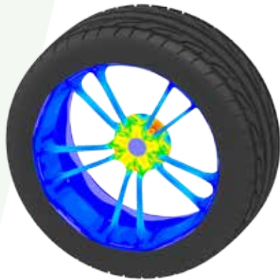
▲ Equivalent stress from sequential bolt pre-tension simulation of an automobile rim Image courtesy SVS FEM.
